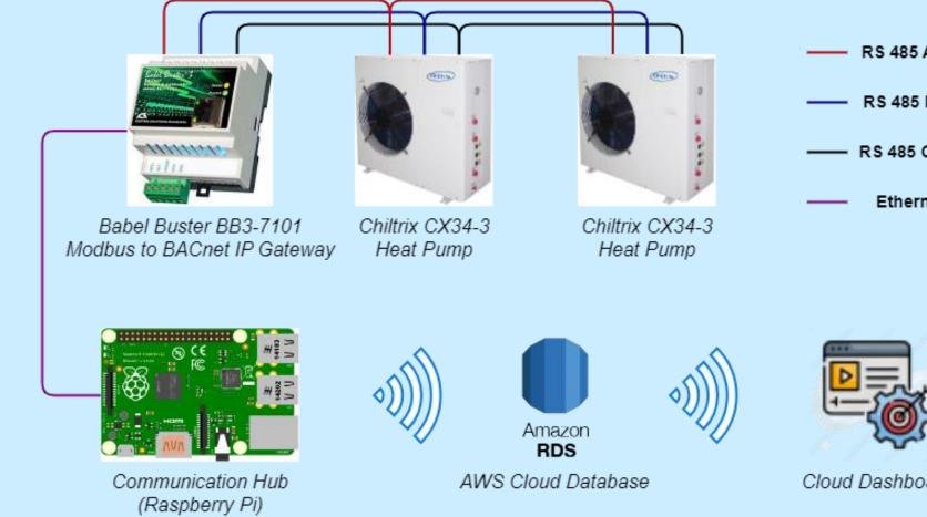
The left figure is the framework of data communication and visualization. The data from heat pumps is aggregated by the gateway through the Modbus-RTU communication protocol. Then all aggregated data is acquired by a local hub (Raspberry Pi) through the BACnet and uploaded to the cloud database. A cloud web application is connected to the database for a user-friendly interface.
