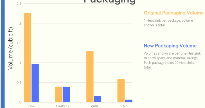
Fig. 4: Difference in volume of packaging components per one heatsink. The total volume saved is 1,328 cubic ft.
