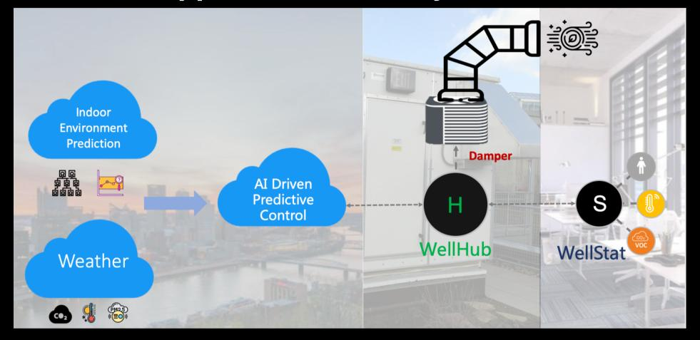
WBC developed an Albased predictive IAQ and energy control solution to optimize the energy consumption and indoor air quality at the same time.
