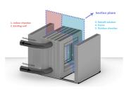
3D visualization of thermal performance testing system
